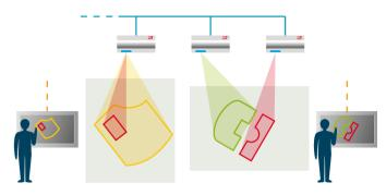
Of course you can show several projection files on several working areas with one installation. The grouping of available projectors is done on request, depending on the size and complexity of the projection.
